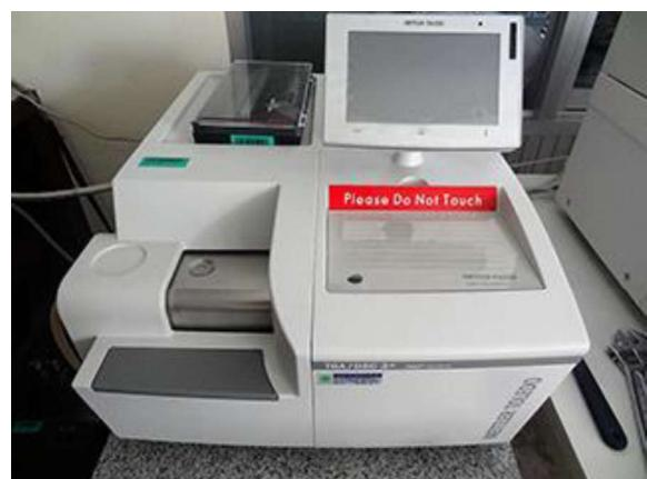
**Thermogravimetric Analysis (TGA)
